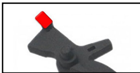
Fig. 5 - Grind or underlay the trigger to prevent the microswitch damage
