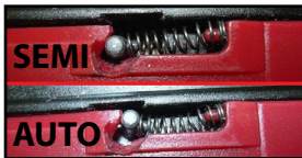
Fig. 3 - selector plate fix for shooting semi fire instead auto
