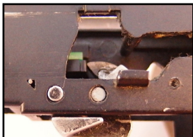
Fig. 6 - Right microswitch press, while is trigger fully pressed
